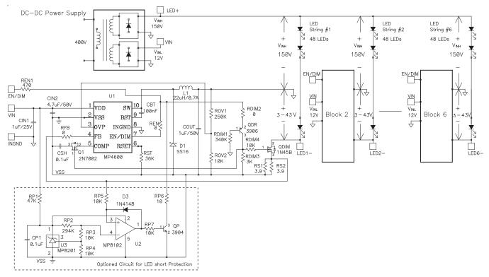
Figure 2—White LED Driver Application for TV Applications
