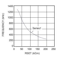
If RSET pin is floating, the setting frequency is the default value 1.35MHz.
